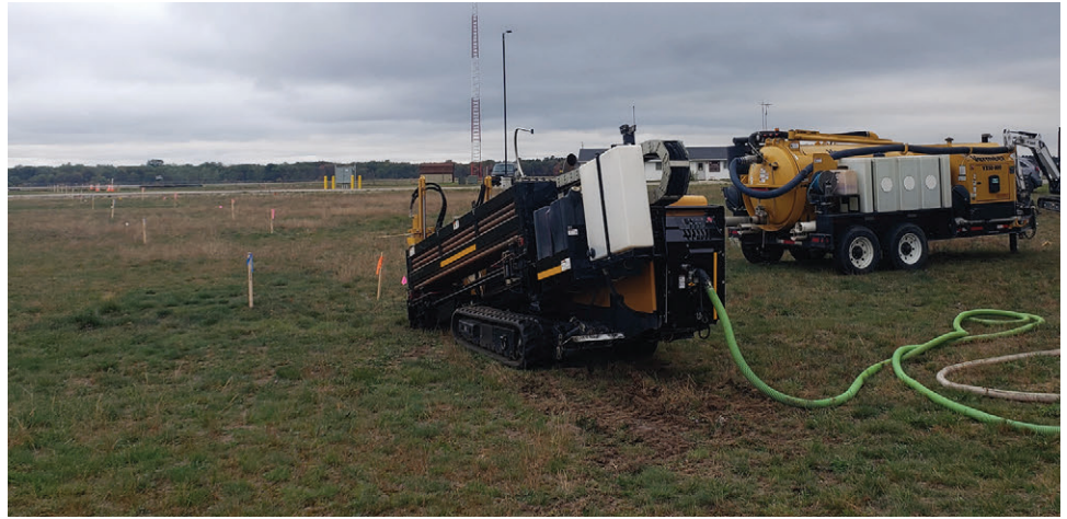
Pre-built Vertebrae well materials are shown in the photo on the left. The directional drilling rig and support equipment are shown in the photo on the right.
