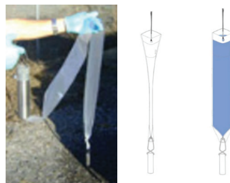
Figure 15: Hydrosleeve™ Passive sampling device.
