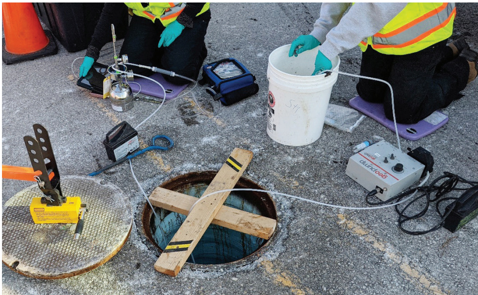
Grab liquid and vapor sampling from a sanitary sewer manhole.
