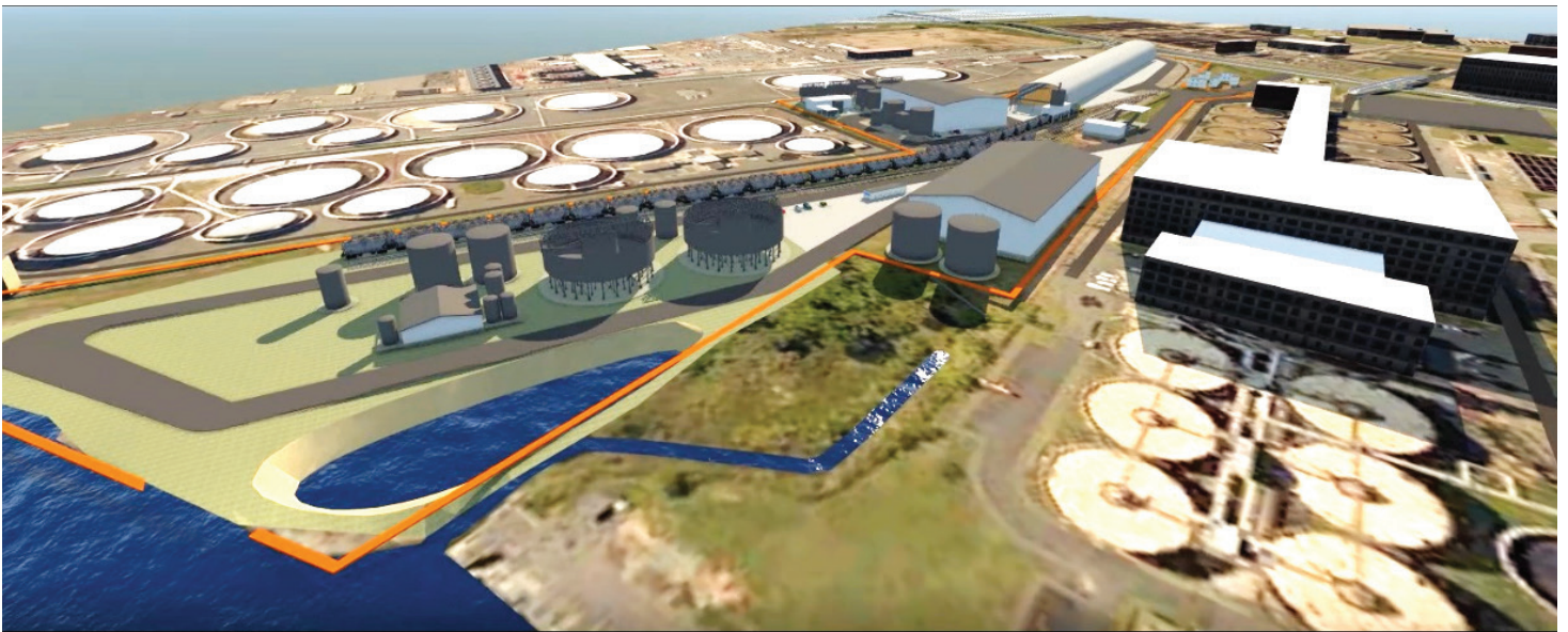
Figure 3: Dredged material processing facility for solids handling and water treatment. The BIM model for this 60% design was created using Autodesk® BIM 360®, Revit®, Civil3D®, Navisworks®, and InfraWorks®. The model is used to visualize how the system fits within the space constraints. Existing aerial imagery was incorporated with the design elements added, bringing the entire project to life. A flyover video of the model was developed to efficiently show the entirety the design. During design development visualization allowed the design team to collaborate seamlessly in the cloud.
