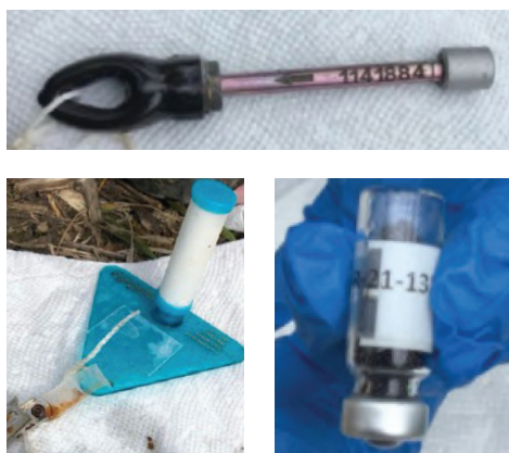
The three different types of passive samplers, ChloroSorber™, Radiello®, and the Waterloo Membrane Sampler™ that were deployed in the sewer during two different sampling events.
